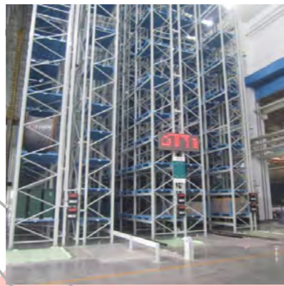
Automatic Storage and Retrieval System
